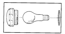
Replace with a 40 watt appliance bulb. Replace bulb cover and reconnect power to range. Reset clock.
