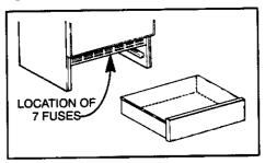
If part of your range does not operate, check to see if a fuse has blown. A gap in the fuse strip or a darkened window indicates a blown fuse. Replace with the same type and amperage type "P" fuse.
