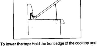
**To lower the top:** Hold the front edge of the cooktop and carefully push back on each support rod to release the notched support. Then gently lower the top into place. The support rods will slide into the range frame.
