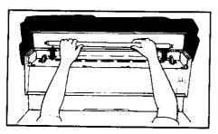
Remove fluorescent tube and replace with an 18 watt fluorescent tube. Snap top trim back into place and restore power. Reset the clock.
